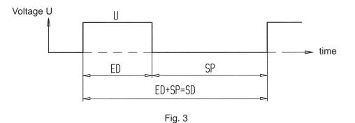
**!! Warning !!** Solenoids with relative duty time have a higher solenoid force than standard solenoids but also greater power consumption. So that the permissible excess temperature limit is not exceeded, these solenoids may only be used for fixed intermittent operation and not for continuous operation.
