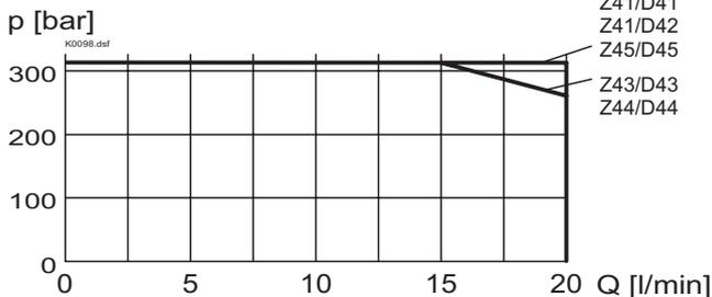
$Q_L = f(p)$  Leakage volume flow characteristics per control edge
