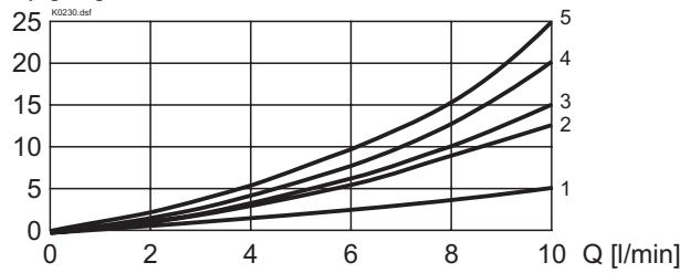
$Q_L = f(p)$  Leakage volume flow characteristics per control edge
