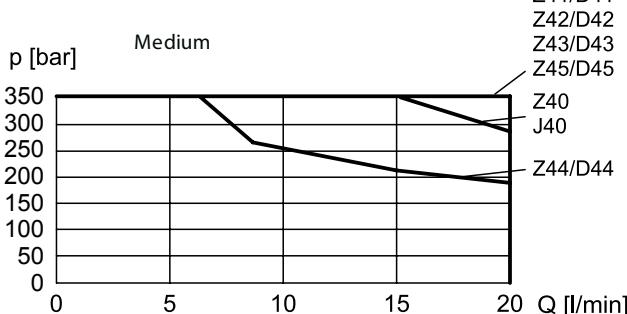
$\Delta p = f(Q)$  Pressure drop volume flow characteristics
