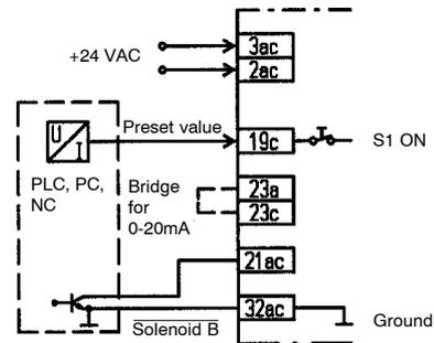
Connection of the preset value module with switch or PLC, PC, NC
