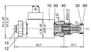
2/2-way version "normally open" [AB] with DIN connector socket
