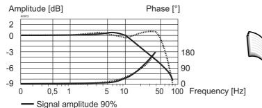
All values measured over 2 metering edges, A and B ports linked.
