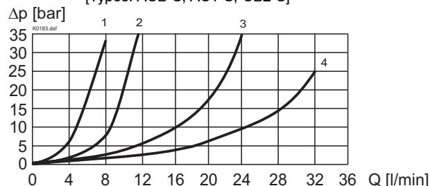
$\Delta p = f(Q)$  Pressure loss/flow characteristics ( $I = I_0$ )
